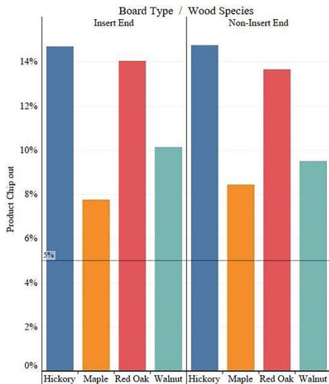
**Figure 2.** Chip-out rates based on wood species and panel types
