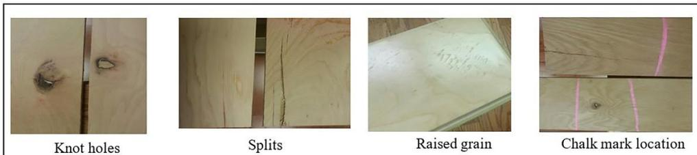
**Figure 10.** Common defects and graders' marking
