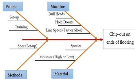
**Figure 3.** Cause-and-Effect diagram listing most probable causes of chip-out
