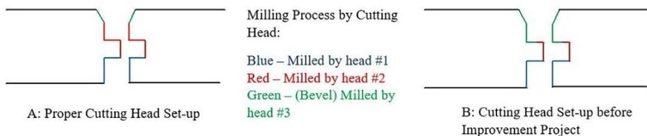
**Figure 4.** Schematic diagram of cutting heads 1-3 milling profile
