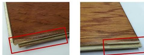
**Figure 1.** Chip-out on the Corners of Flooring
