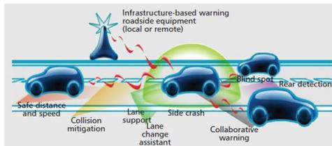
**Figure 3.** Intelligent vehicle to infrastructure communication (Nkoro & Vershinin, 2014)
