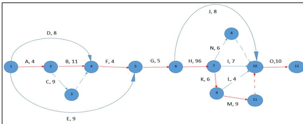
**Picture 3.** Technological-organizational structure of a process occurring in one operating room within one working day with the critical path (red) – PERT method, expected times.
