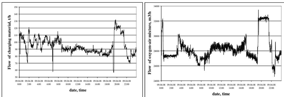
Figure 2. Change of parameters of loading of the Vanukov furnace during one day
