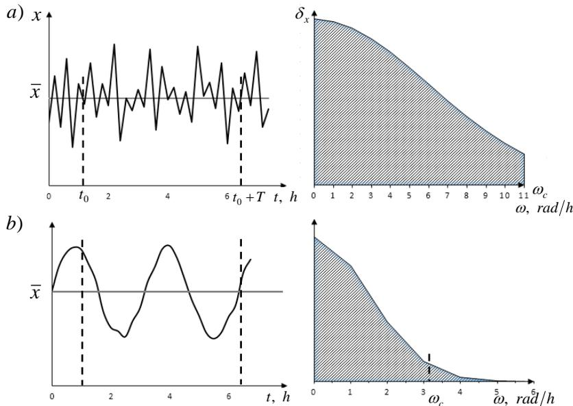
**Figure 1.** High-frequency (a) and low-frequency (b) oscillations (left, - changing in time, right - spectral density)
