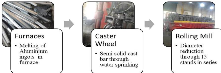
Figure 1. Rolling mill process flow
