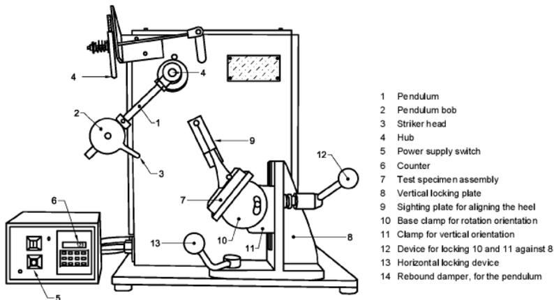
**Figure 3.** Fatigue-testing apparatus (ISO 19956)
