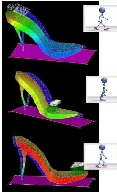
**Figure 13.** FEM simulation of shoe and heel strain reactions under simplified load conditions
