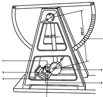
**Figure 2.** Lateral impact tester (ISO 19953)
