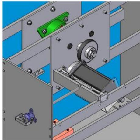
**Figure 8.** Pendulum releasing system
