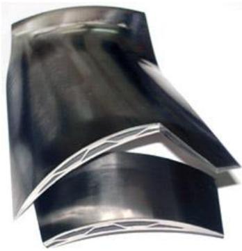
**Figure 4.** Hollow wide chord fan blade
