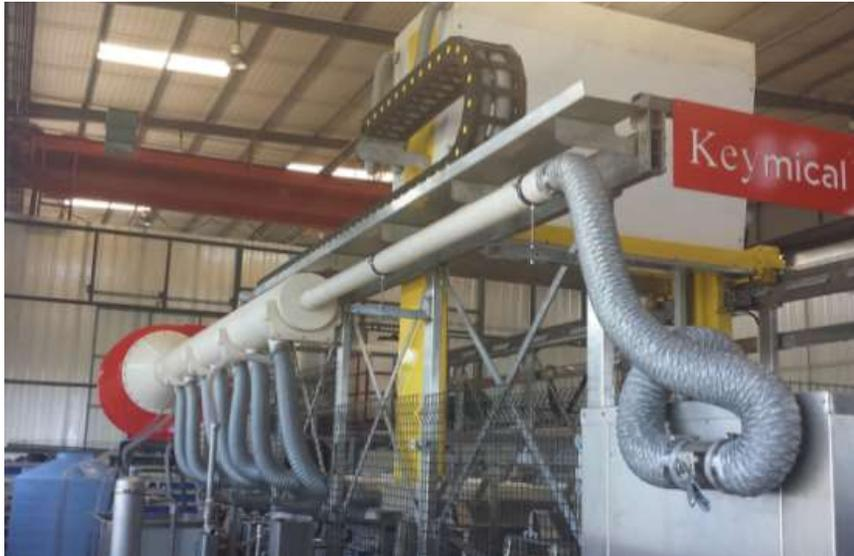
**Figure 23.** Example of Injection Mould Ultrasonic Cleaning Machine with a multi stage treatment (Courtesy of Keymical)
