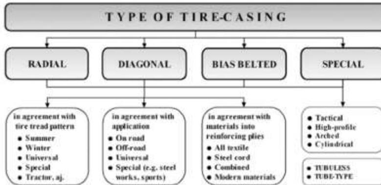
Figure 5. Type of tire-casing (Košťál et al, 2012)
