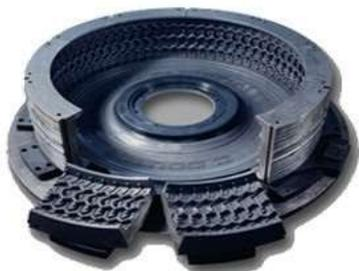
**Figure 12.** Tire mould [Courtesy of Tianyang Mold Co., Ltd]
