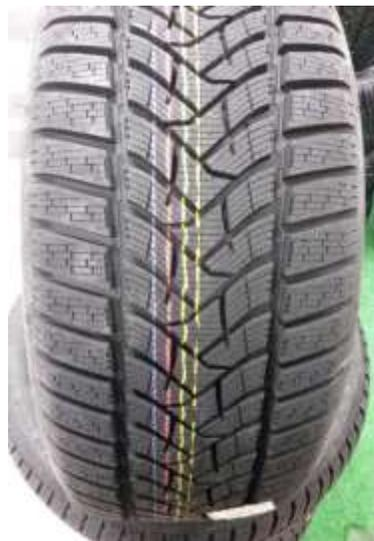
**Figure 15.** New tire with colored stripes for tread's identification
