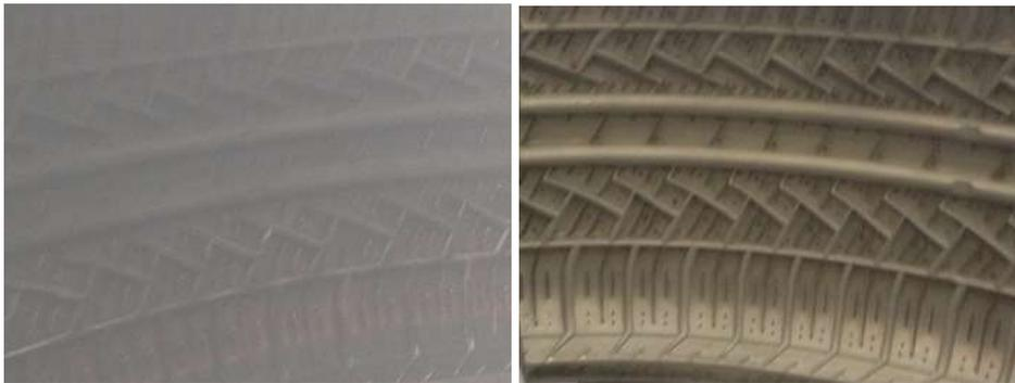
**Figure 24.** Comparing tire surfaces before and after the Injection Mould Ultrasonic Cleaning (Courtesy of Keymical)
