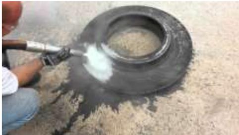
**Figure 18.** Sandblasting of a sidewall [Courtesy of Eco Blast]
