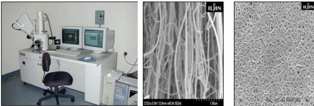
Figure 2. SEM apparatus and images
