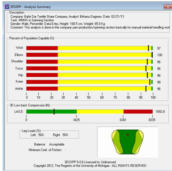
**Figure 9.** Software analysis for male operator posture (an acceptable posture)
