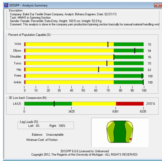
**Figure 11.** Software analysis for female operator posture (an acceptable posture)
