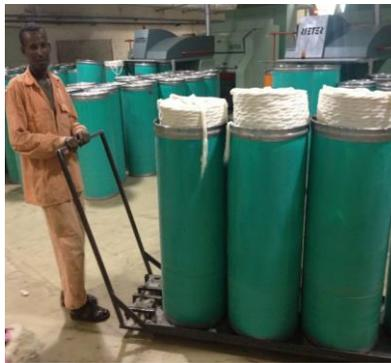
**Figure 13.** Small push or pull to MMH equipment for faster movement
