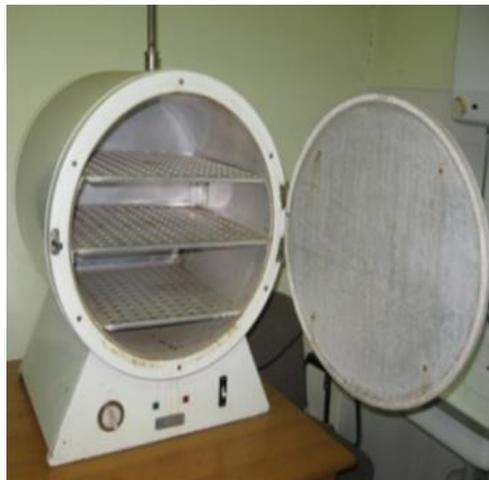
Figure 7. Laboratory dryer
