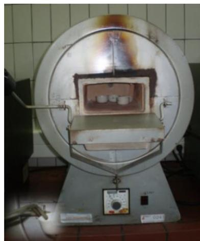
**Figure 8.** Electric furnace, cups and metal tongs
