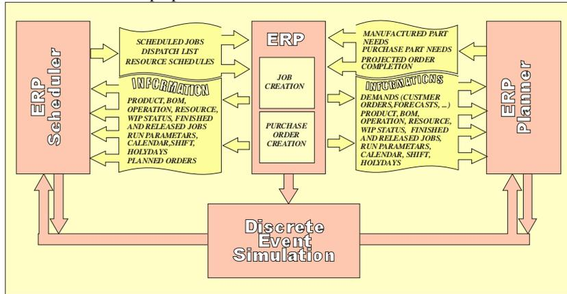
Figure 2. Closing the Planner/Scheduler Loop with simulation
