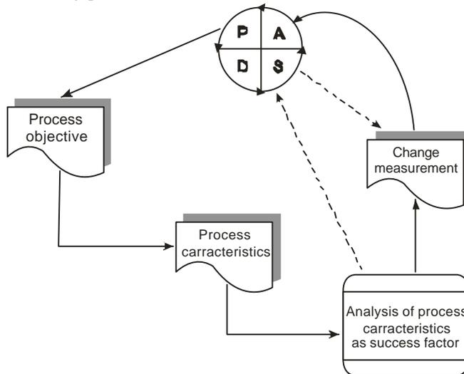
Figure 1. Process quality improvement procedure
