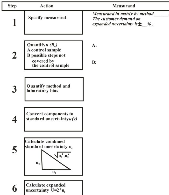
Figure 3 - Flow scheme for calculations measurement uncertainty
