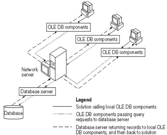
Figure 8. Client server architecture
