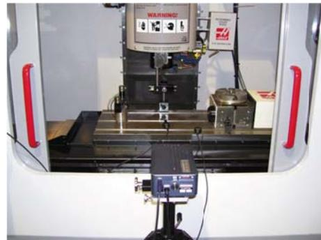
Figure. 3 Measurement using Laser interferometer
