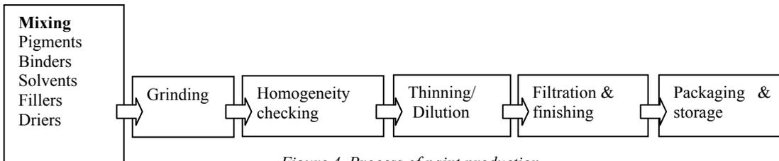
Figure 4. Process of paint production
