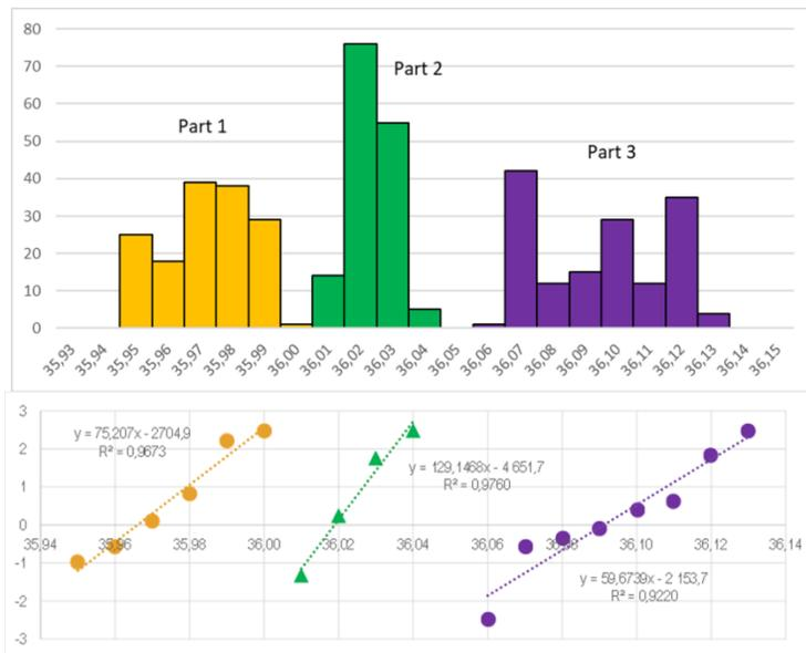
Figure 2. Histograms and empirical DFs for many repeated measurements
