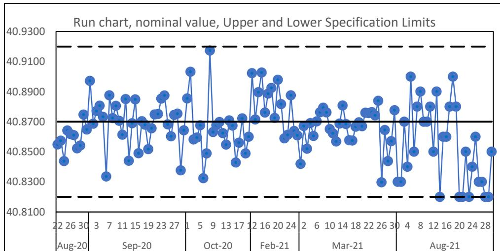
Figure 5. Run chart for the hole  $\varnothing 40,87 \pm 0,05$
