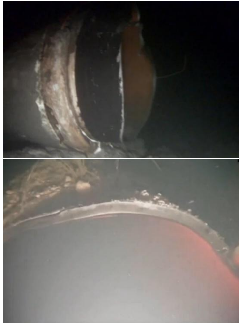
Figure 6. Destruction of the Nord Stream-1 pipeline section, initial inspection results
