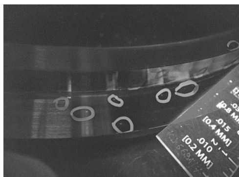
Figure 2. The porosity on the mechanical seal
