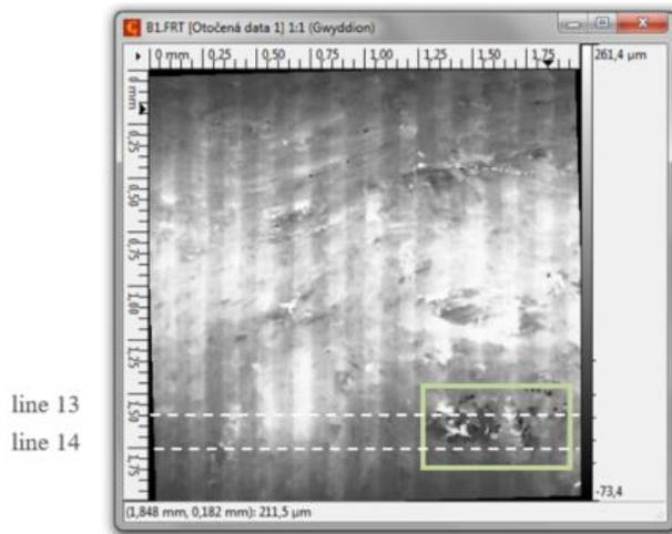
**Figure 14.** Scanned area (size: 2x2 mm) – highlighted area crossing line 13 and 14
