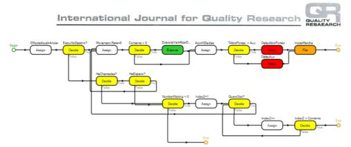
Figure 2. Process responsible for deciding an elevator stop
