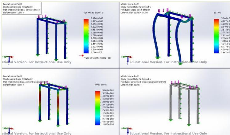
Figure 11. Simulation of the main structure in wood. (Developed by author's own method)
