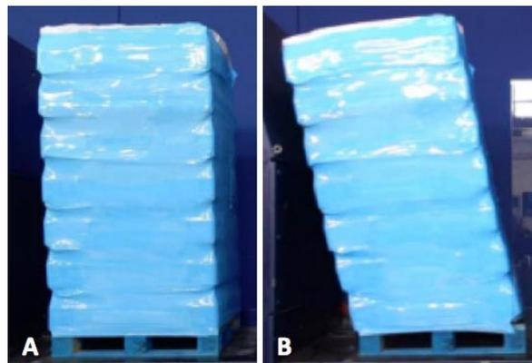
**Figure 1.** Pallet at rest (A) and accelerated (B). Example of load unitized by stretch wrap: even though the pallet is subjected to an acceleration, the stacked packs of bottles depicted a single-body behavior (Fragassa et al., 2017).
