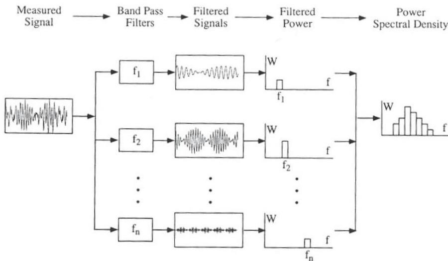
**Figure 5.** Spectral analysis procedure using analog filter (ANSYS inc. 2009)
