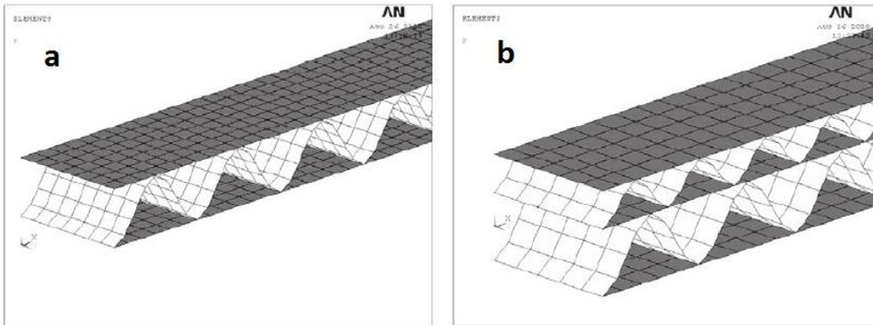
**Figure 9.** (a) Single-wave paperboard, (b) Double-wave paperboard (Park et al., 2012)
