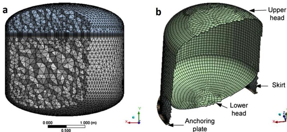
**Figure 4.** (a) fluid domain mesh, (b) view of the tank FE model (Nicolici & Bilegan, 2013)
