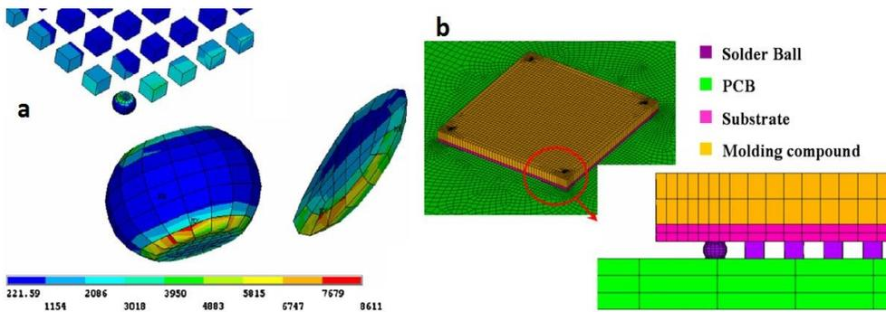
**Figure 7.** (a) Equivalent stress distribution on solder balls, (b) 3D finite element model of the BGA package (Yu et al., 2011)
