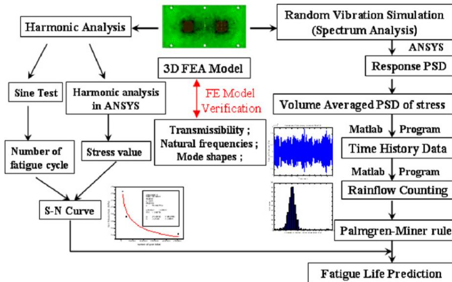
Figure 6. High-cycle fatigue life prediction (Yu et al., 2011)
