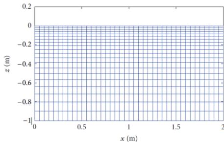
**Figure 3.** A mesh composed by isoparametric four-noded elements (Kolukula & Chellapandi, 2013)
