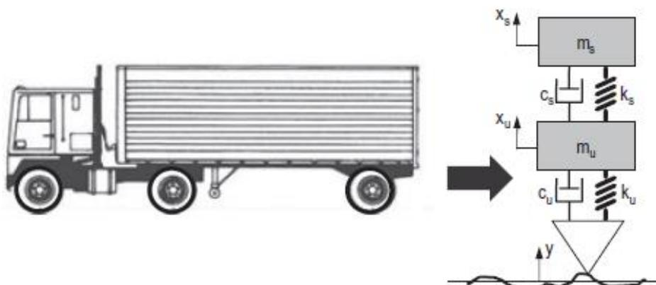
**Figure 8.** Schematic of two degrees of freedom quarter-car vehicle model (Rouillard, 2008)
