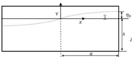
**Figure 2.** Sloshing of liquid in a rectangular tank (Goudarzi & Sabbagh-Yazdi, 2012)
