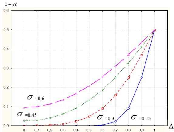
**Figure 3.**  $\sigma$  and  $\Delta'$  effect on the defective items fraction ( $1 - \alpha$ )
