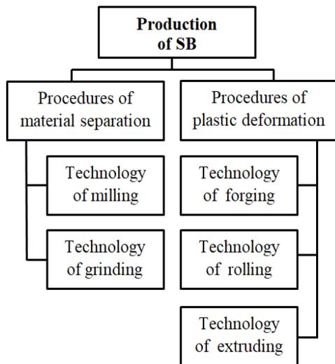
**Figure 1.** Procedures of the SB making
