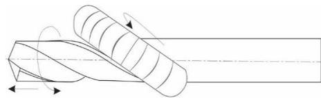
**Figure 2.** Making of a drill bit groove by milling technology
