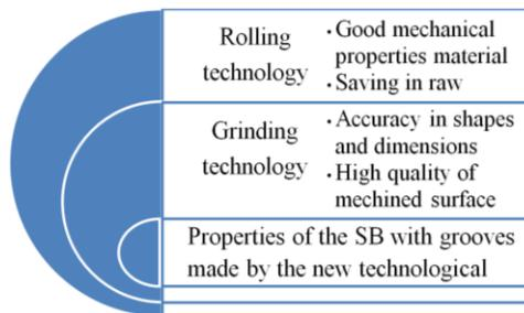
**Figure 9.** Properties of a groove with a groove produced by a new technological process
