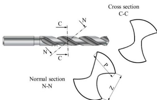
**Figure 11.** Cross section and the normal section of the SB
