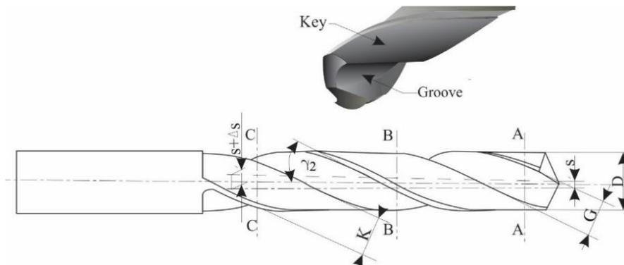
**Figure 10.** Geometric elements of the SB groove
