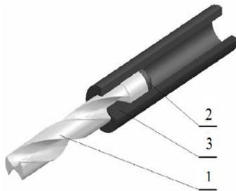
**Figure 5.** Making of SB groove by extrusion: 1 – SB, 2 –material, 3 – matrix (Bulzak & Pater, 2013)
