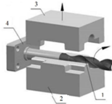
**Figure 6.** Making of a SB groove by extrusion in a two – part mould: 1 – SB, 2 – lower part of the mould, 3 – upper part of the mould, 4 – extruder (Bulzak et al., 2014)
