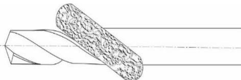
**Figure 3.** Making of a drill bit groove by grinding technology
