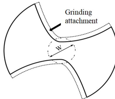
**Figure 8.** The scheme of SB groove making by a new technological procedure
